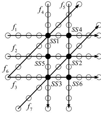
Fig. 3. Evaluation Scenario with seven flow, three 3-flow star-structures, and three 2-flow star-structures.
