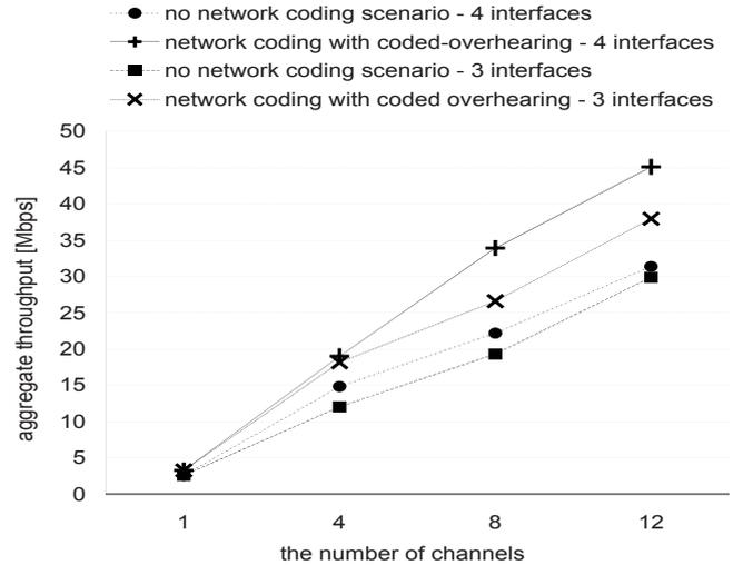
Fig. 4. Aggregate throughput in the no-coding scenario and the network coding with the coded-overhearing scenario.
