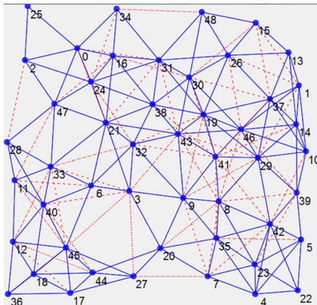
**Fig. 4** The mesh network topology used for evaluation consisting of 49 nodes randomly located in a square of size  $7 \times 7$ . The communication/interference range are equals to 1.7 and 2. The *solid/dash lines* illustrate the node-pairs which are in communication/interference range of each other
