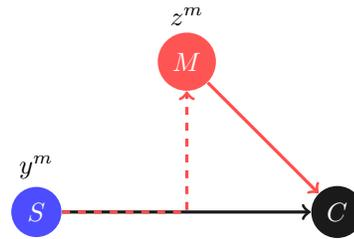
Fig. 1. Illustration of network compression via overhearing helper  $M$ . The memorized sequence  $y^m$  represents the total past data from  $S$  to the clients overheard by  $M$ . The overhearing channel is represented by dotted line.
