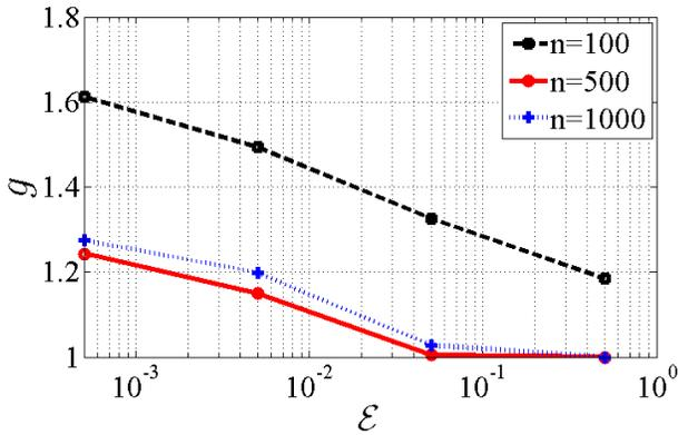
Fig. 3. Gain of memory-assisted compression over the end-to-end compression. The memory size is  $m = 10^6$ .
