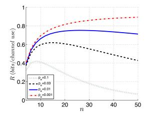
Fig. 5. Optimal code rates versus the code length for different values of  $p_e$
