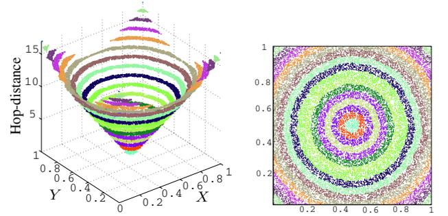
Fig. 10. Illustration of occurrence of annuli in a network with  $n = 25000$  and  $r_n = 4r_n^*$ .
