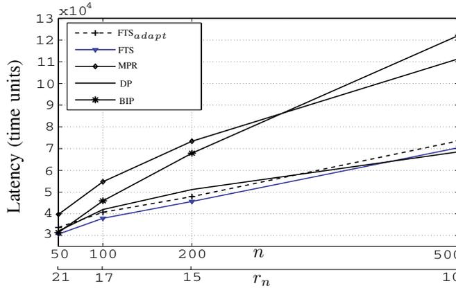
Fig. 7. Latency of different schemes for broadcasting 2000 packets over a random network.
